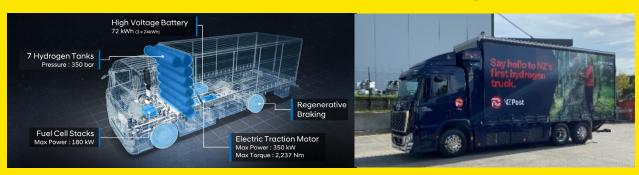
Our Hydrogen Fuel Cell Electric Vehicle, also known as an FCEV, ticked over 100,000 km last month. An FCEV converts the chemical energy of hydrogen gas stored in the onboard tanks and oxygen from the air into electricity by passing through a fuel cell, which is then used to power the electric motor propelling the truck.
