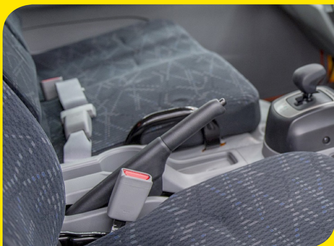
Typical handbrake lever of Cardan Shaft park brake equipped truck. You will notice the “ratchet” type feel.
