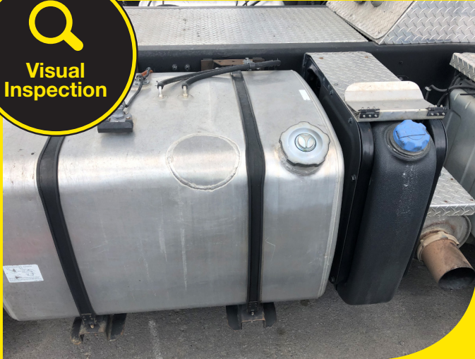
Diesel tank and filler (left). AdBlue tank and filler (right). Special care needs to be taken to not mix these up.
