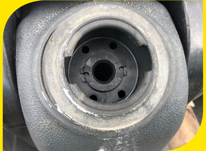
Inside the AdBlue filler, there is a restrictor, as AdBlue pumps are narrower than diesel pumps. This should prevent a diesel pump filling the AdBlue tank.
