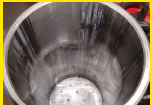
Figure 2 - Scored cylinder liner caused by a build-up of carbon on the piston due to high idle time.
