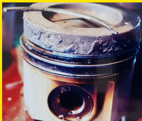
Figure 1 - Piston with excessive carbon (soot) build-up and a broken piston ring.
