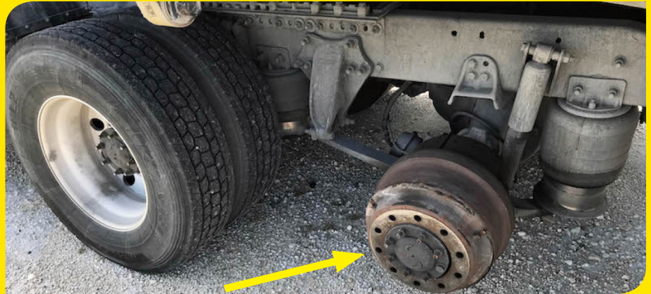
This is the end result of when a retorque is not completed. We do not want to see this.
