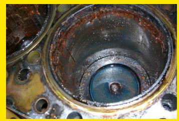
This is damage to a hydraulic pump after it ran on fluid heavily contaminated with diesel fuel. The pump, cylinder, and other components needed replacing as well as a major system clean-out, resulting in lengthy downtime.
