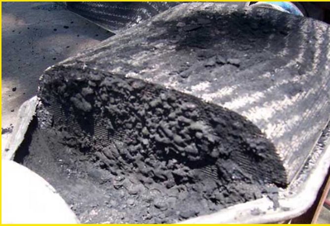
This is an example of a severely blocked diesel particulate filter.
