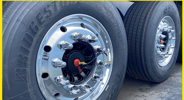
The TPMS air supply line from the axle tube to the tyre.
